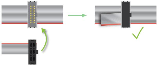
Next, make sure your module's power cable is properly connected to your module. For 2hp modules, confirm that your cable's red stripe aligns with the white marker line on the module's PCB, just above the power header. You may notice that even though there is only 1 row of 5 pins on your 2hp module, but 2 rows on the power cable. You can use either row of 5 pin connectors on the cable with your module, so long as the red stripe is properly aligned. See figure below for reference:
